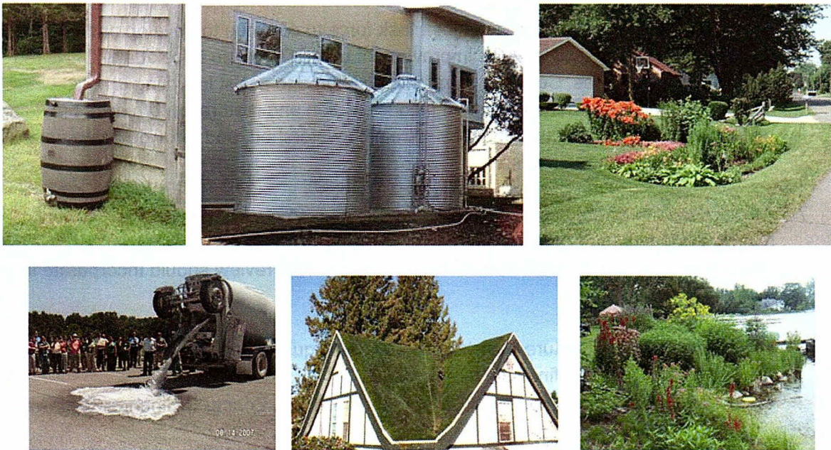
Figure 16: Voluntary, Site-level Stormwater Management Techniques (rain barrel, cistern, rain garden, porous concrete, green roof, shoreland vegetative buffer)
